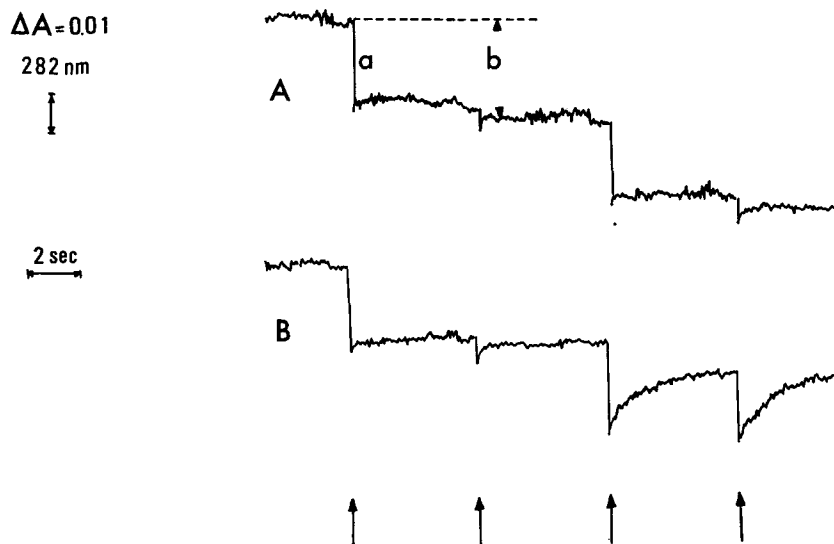
Fig. 4. Light-induced absorbance changes observed at 282 nm. Excitation: laser flashes spaced 5 s apart as indicated by the arrows. Reaction center concentration 2 \mu\text{M} in 0.3 % LDAO, 0.1 M Tris \cdot HCl, pH 7.5, in the presence of 25 \mu\text{M} ubiquinone. The electron donor was reduced cytochrome c : 25 \mu\text{M} for trace A and 5 \mu\text{M} for trace B.
